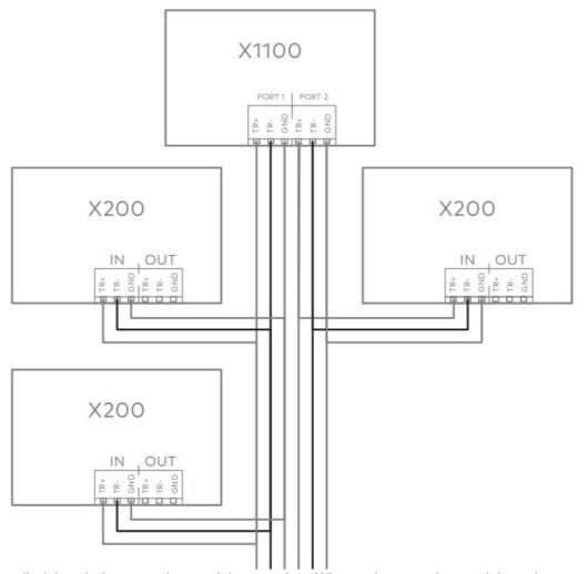
For ease of install, daisy chain expansion modules together. Wire each expansion module to the next module instead of wiring directly back to the controller.
