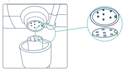
Hold the black plug and insert it into the hole. We have set up corresponding raised parts and recesses for proper alignment.
