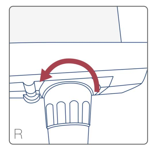
Tighten the other end in the same manner by turning counter clockwise.
