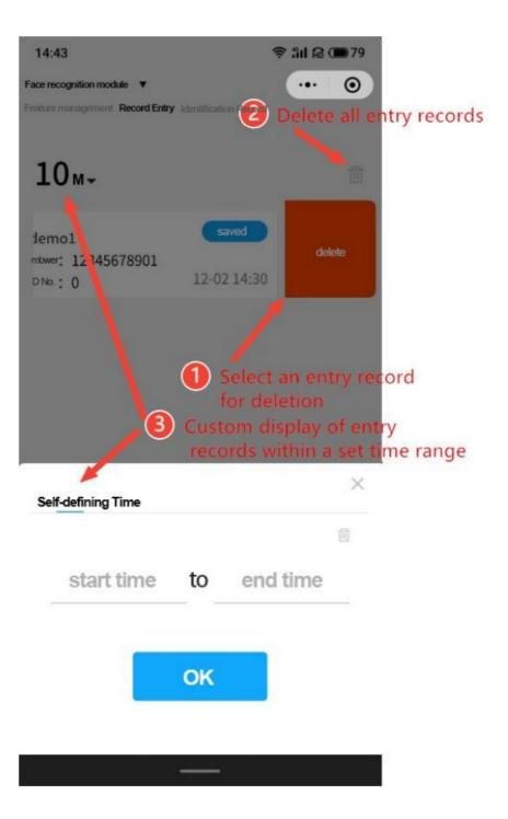
Identification record interface (display/record of records triggered by successful identification at the device end):
