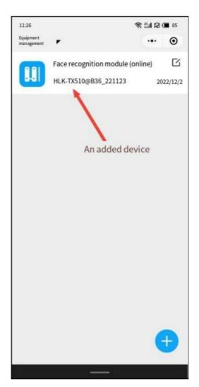
5. Click the newly added device to enter the feature management interface to add feature values. When adding the first feature value, directly click the function button of "Add Feature" in the middle, and enter the portrait photo, name and mobile phone number to be added. After the input is complete, click the "upload now" function button below to add the face information to the device;
