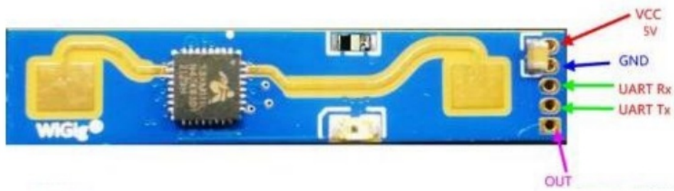
Figure 6 Module pin definition diagram
