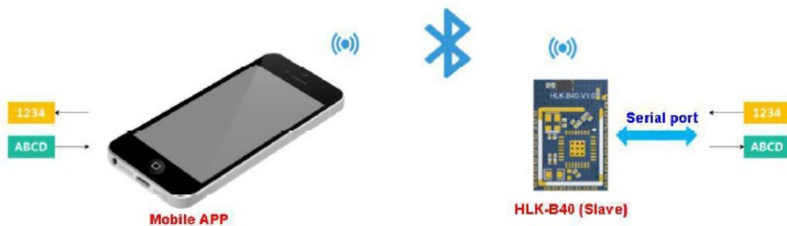
Figure 4 One-to-one Bluetooth connection transmission function schematic
