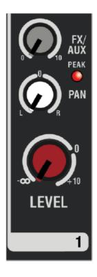
**NOTE:** When not using a channel, it is recommended to keep the level knob at  $-\infty$  to keep noise to a minimum.
