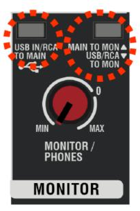
• The two buttons highlighted in the image on the right can be used to direct the USB/RCA bus to various outputs. Use the lefthand button to route the USB input to the Main bus and the righthand button to route the USB input to the Monitor/Phones outputs.
