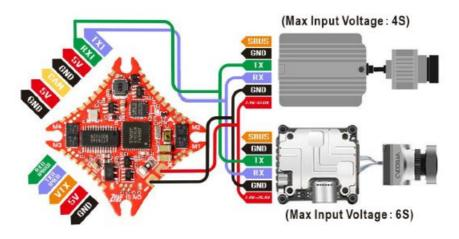
2. VTX serial port opens. The protocol is selected according to its own VTX protocol.
