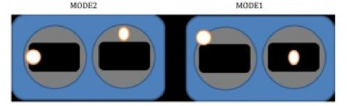
The graphics above show the stick command to bring up the OSD menu. The stick command is: throttle centered, yaw left, pitch forward. The exact stick command therefore depends on which mode your transmitter sticks are in. In the OSD menu, use pitch up/down to move the cursor between menu items. When a menu option has a > symbol to the right of it, this indicates that it contains a sub-menu.
