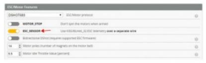
2. Open ESC telemetry serial port. TX on the ESC needs to be connected to the RX6 on the flight controller to use the ESC telemetry
