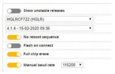
6. Click Load Firmware [Online] Load firmware. Flash Firmware Waiting for completion
