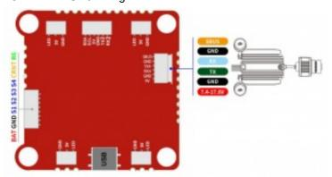
3. 5.8G VTX serial port opens. The protocol is selected according to its own VTX protocol.
