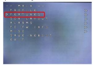
Roll-right will enter the sub-menu. For example, in the screen to the right, moving the cursor to "Features" and then moving the roll stick to the right will enter the "Features" sub-menu.
