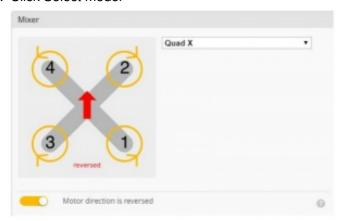
2. Click "I understand the risks" Push Master to check motor steering "Master" Steering can be changed at BLHeliSuite
