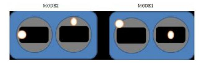
The graphics above show the stick command to bring up the OSD menu. The stick command is: throttle centered, yaw left, pitch forward. The exact stick command therefore depends on which mode your transmitter sticks are in. In the OSD menu, use pitch up/down to move the cursor
