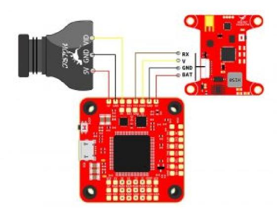
2. VTX serial port opens. The protocol is selected according to its own VTX protocol.
