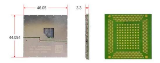
31PHBM2000A is a smart automotive LTE module, which is designed by FIH, with strictly follow IATF 16949:2016 global technical specification and quality management standard for automotive industry. This NAD module could afford harsh environmental tests and has superior performance for ESD and EMC. It is a solution designed specifically for automotive industry, on intelligent connected vehicle application field.
