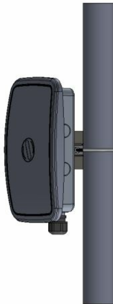
Figure : Final alignment of 2x2 outdoor AP and mounting bracket
