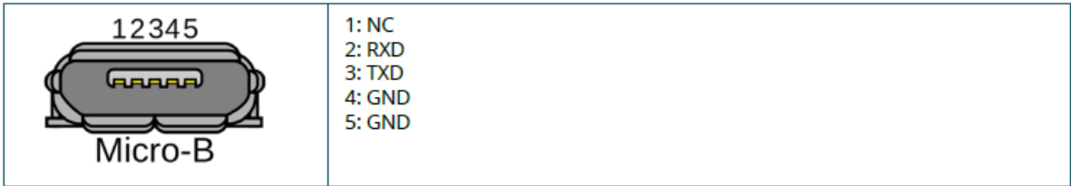
Figure 6 Micro-B Console Port Pin-out
