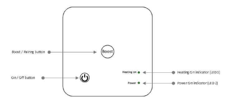
Pressing the BOOST button once with the power on will turn on the heating for 15 minutes regardless of T2 or App temperature settings. Pressing BOOST twice will turn it on for 30 minutes; three presses for 45 minutes and four presses for 1 hour.
