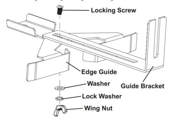
2. Loosen the Guide Locking Knob. The short end of the Edge Guide should slide underneath the Guide Locking Knob. Align the Edge Guide to the mounting position of the Base Plate and insert it to the desired working height.
