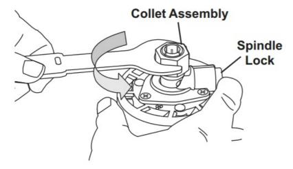
10. Insert at least 3/4 of the shank end of the new router bit (sold separately) into the opening in the Collet Assembly.
