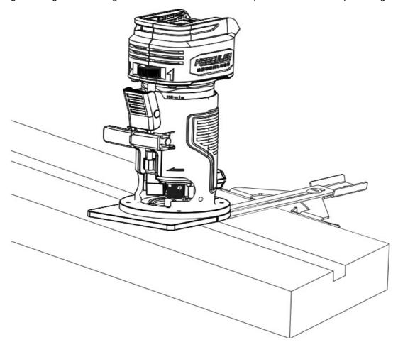
**Note**: The Edge Guide may be used for circle cutting by turning the Edge Guide over and using the center gap in the Edge Guide to follow the circle.
