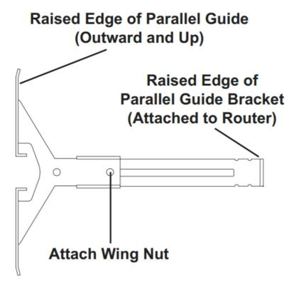
3. Align the Edge Guide along the temporary guide secured to the workpiece to cut parallel with the temporary guide.
