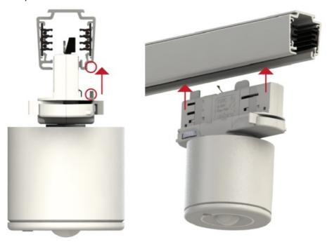
2. With the rib in its allocated groove, ensure the securing lever (located on the opposite side to the rib) is fully pressed against the underside of the track.
