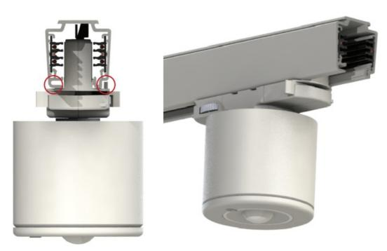
3. Use the locking levers at each end of the adapter to secure the Tracksensor in place. The unit will be fully fitted when both levers 'click' and are parallel to the track. Ensure the Tracksensor sits flush to the track.
