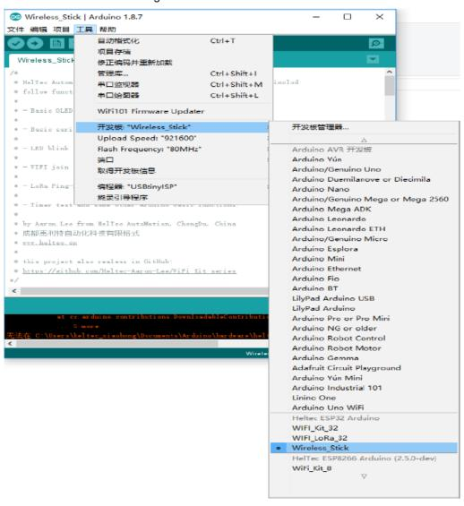
You can find the board Arduino routines for various resources in the "Examples" menu, which you can compile directly and download to your WIFI Kit development board. Attention to the corresponding development board model, choose the wrong model may lead to compile errors. As shown in Figure 2-2:
