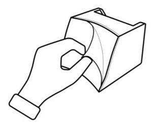
Installation with heat gun application. Peel off the plastic cover of the tape and apply heat with a heat gun (not included). Wait for the tape's surface to heat up. Place the mount on the helmet's appropriate surface. Continue with **Step 3.**
