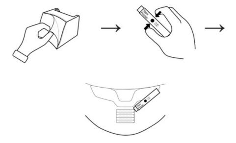
**Step 3**. Apply pressure for at least 1 minute towards the helmets surface and release. Note, follow Table 1  $\rightarrow$  Application  $\rightarrow$  None / Heat / Tape Primer (page 6), to know the appropriate times to leave the mount resting in order to ensure proper adhesion between the mount and the helmet.
