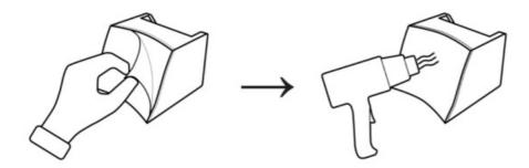
Installation with tape primer application. Peel off the plastic cover of the tape. Grab the tape primer (sold separately) and apply pressure on the dot location indicated as "Crush at dot" on the tape primer until it breaks. Apply a single coat of the primer on the helmet's appropriate surface. At time of application, make sure the room temperature is  $60^{\circ}F - 80^{\circ}F$  ( $15^{\circ}C - 27^{\circ}C$ ). Place the mount on the helmet's appropriate surface. Continue with **Step 3.**
