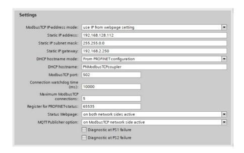
**ModbusTCP IP-address mode:** Setting the IP address for the ModbusTCP network. Selectable are "DHCP", "Static IP", "use IP from the web page setting".
