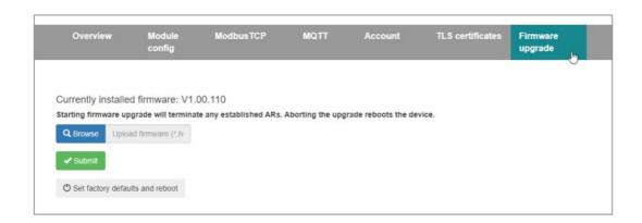
With the button "Browse" the firmware can be selected. With the button "Submit" the firmware is transferred to the PN/ModbusTCP coupler and burned. Afterwards the PN/ModbusTCP coupler executes a reboot, and the new firmware is active.
