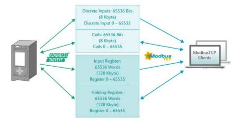
From the point of view of ModbusTCP communication, all coils, inputs and registers are always available in the PN/ModbusTCP coupler. So it is always possible to access all data types from address 0-65535. Via the PROFINET configuration the ModbusTCP data can be assigned to the PLC I/O image in the slots, which are required in the PLC program. Up to 300 slots are available in the PN/ModbusTCP coupler for such assignments. The following modules are available to access the ModbusTCP memory:
