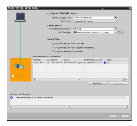
The unique identification of the PN/ModbusTCP Coupler in the PROFINET network is guaranteed by the MAC address of the device. The PROFINET MAC address can be read on the front panel of the PN/ModbusTCP coupler on the left side at X1 ("MAC 1").
