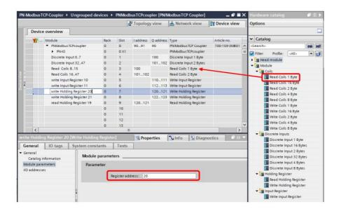
All modules have as **parameter** the **register number** (Input Register, Holding Register) or the first **bit address** (Discrete Inputs, Coils). For the Input Bits and Coils from 8 bits (1 byte) up to 256 bits (32 bytes) can be addressed together in one slot.
