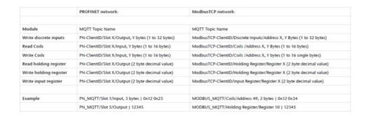
On both network interfaces the following MQTT topics can be read additionally:
