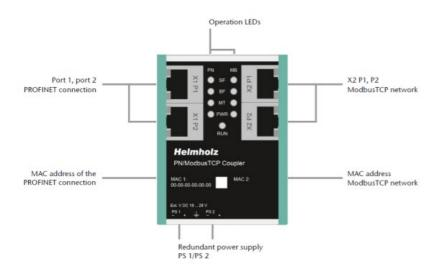
The housing of the PN/PN Coupler is not grounded. Please connect the functional earth terminal of the PN/PN Coupler properly to the reference potential.
