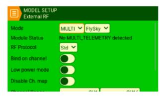
Press and hold the MDL button and scroll to the MODEL SETUP page. Under internal RF, set the Mode to MULTI and select the RF Protocol/ sub protocol as desired. Once the protocol is selected, the corresponding RF chip will be activated.
