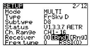
Press and hold the MDL button and scroll to the MODEL SETUP page. Under internal RF, set the Mode to MULTI and select the RF Protocol/ sub protocol as desired. Once the protocol is selected, the corresponding RF chip will be activated.
