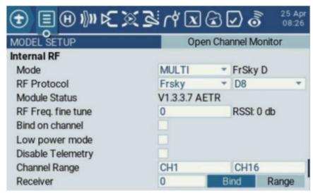
Press and hold the MDL button and scroll to the MODEL SETUP page. Under internal RF, set the Mode to MULTI and select the RF Protocol/ sub protocol as desired. Once the protocol is selected, thecorresponding RF chip will be activated.
