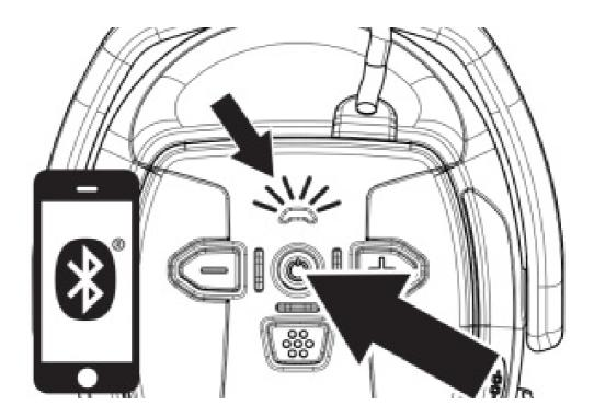
ON – Hold down the button until the LED flashes BLUE. (automatic connection to the paired phone after 1st pairing)
