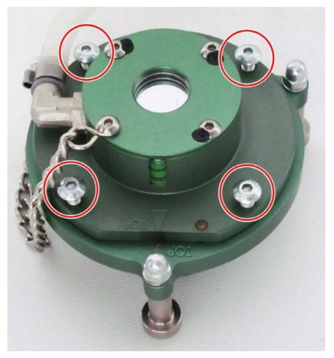
3. Insert the hose of the adjusting device inside the hose of the manual vacuum pump. Only insert the hose partially, as the hose will contract due to the vacuum.
