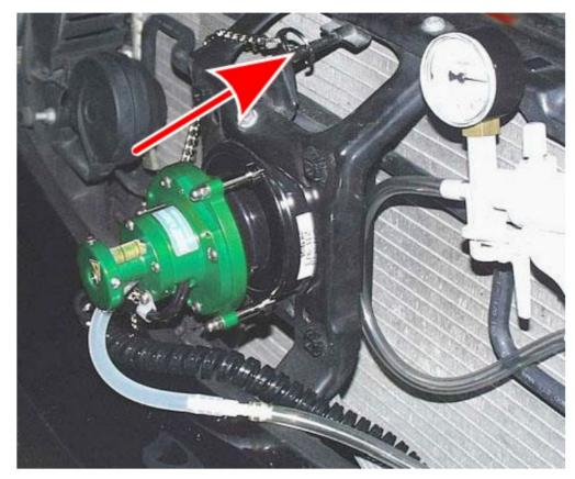
7. Position the vacuum bell over the radar head.
