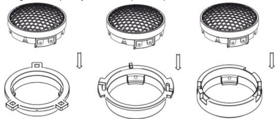
The optionally available car-specific tweeter adaptor rings allow a tailored and acoustically optimized adaption of the HELIX COMPOSE tweeters to the vehicles original mounting location.
