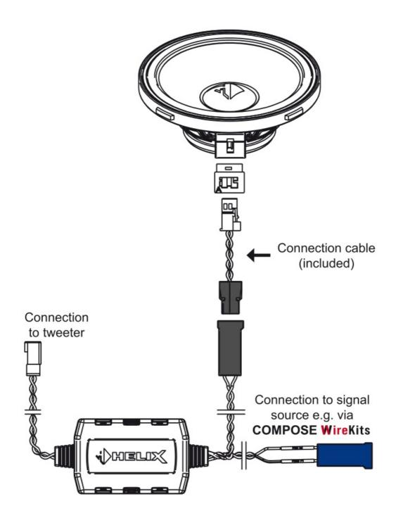
Option d: Direct connection to OEM connector with optionally available FlexConnectinlay
