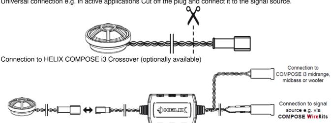
Ensure that all components are correctly connected (phase), i.e. plus to plus and minus to minus. The positive leads of the loudspeaker system are marked with a red stripe.
