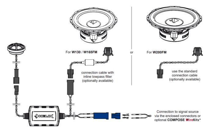
Ensure that all components are correctly connected (phase), i.e. plus to plus and minus to minus. \*Contact your retailer or visit www.audiotec-fischer.com/compose for an up-to-date overview of available COMPOSE **WireKits**.
