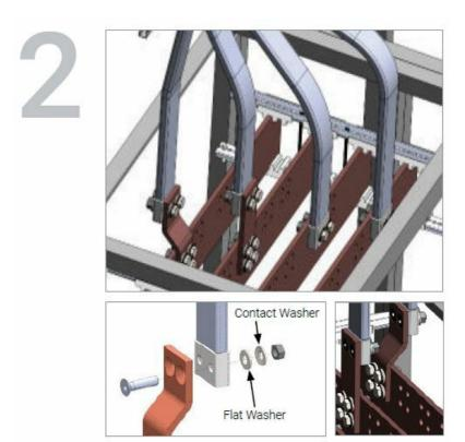
Connect the ready-to-use FleXbus conductor with pre-punched holes to the switchboard. This connection can be made directly onto the busbar or circuit breaker with optional palm extenders
