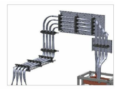
Install conductors into the supports and mount the top part of the supports. Leave excess conductor length at the top of the transformer/power supply.
