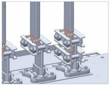
Connect FleXbus conductor with HCBC clamp and plate
