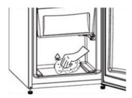
After defrosting is complete, clean the inside of the appliance with a solution of warm water and a little bicarbonate of soda, then dry thoroughly. Wash all removable parts in the same way and reassemble. Reconnect the appliance EN – 20 to the mains supply and leave for 2 to 3 hours on setting number '5' before introducing the food back into the freezer.
