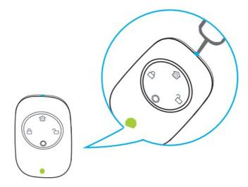
According to APP prompt, press the button for 2 seconds, green LED flash quickly, APP Interface prompted, networking success. (Press networking hole for 5 seconds if any changes for internet, green LED flash slowly for 3 seconds, exit network successfully.
