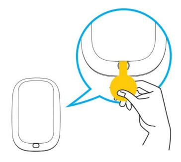
• Remove battery insulation film to power on
