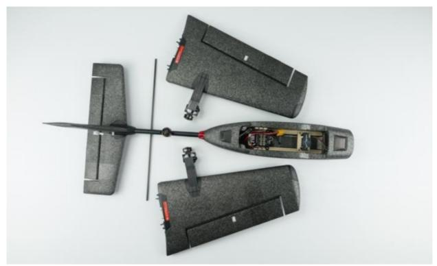
$\bullet\,$  y. Slot the carbon rod into the main wing.
