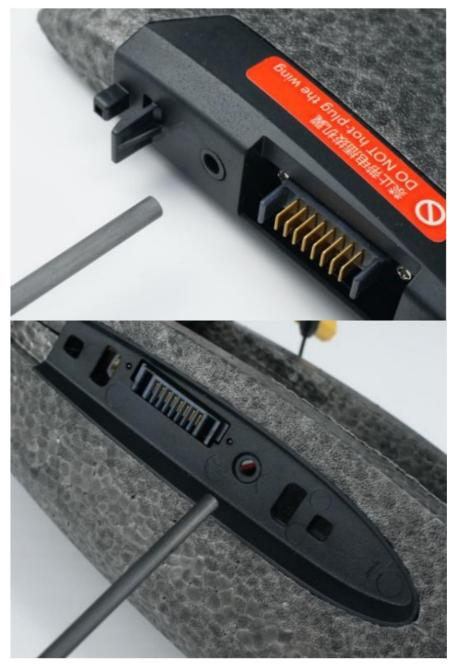
• z. Carefully attach the main wing onto the fuselage and ensure that it's properly clipped onto.
