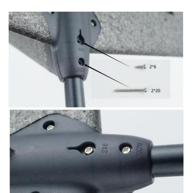
• g. Now let's assemble our completed tail onto the main fuselage. This is to be secured with the provided nut.
