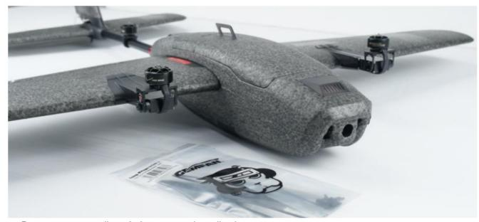
• ag. Prepare your propellers, 2×8 screws and an allen key.
