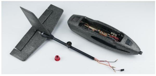
• h. Slot the red color nut onto the tail boom first, and observe the direction as shown below.
