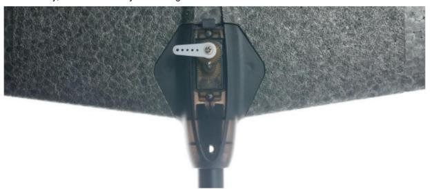
• e. Align the vertical stabilizer onto the clip of the horizontal stabilizer as shown below and install it.
