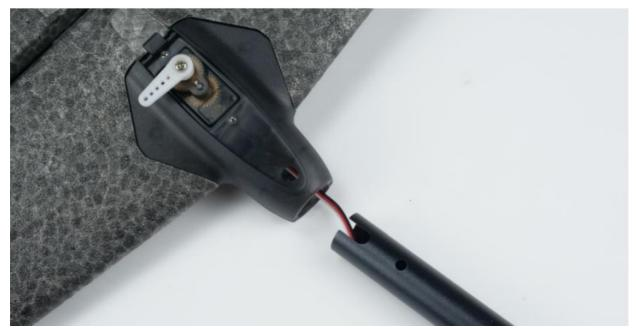
• **d.** After inserting the tail boom, ensure the U-shaped cut is centered and is not pushing onto any wires. If installed correctly, the hole is clearly see through and the servo wire is visible as well.
