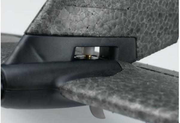
• f. Rotate to the other side and install the corresponding screws according to the marking on the mount.
