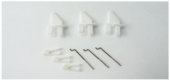
• p. After installing the steel linkage into the latch, place it in the opening of a vernier caliper, the end-to-end length should be 46mm. If you do not have a vernier caliper, you may use a ruler. Repeat the same thing for the other 2 linkages.
