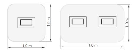
• Curing area at 55 cm distance for IRT UVA-1 is 1,0×1,0 m (HxW) with a UV-A intensity of 25W/m<sup>2</sup>. Curing area at 55 cm distance for a IRT UVA-2 is 1,0×1,8 m (HxW) with a UV-A intensity of 25W/m<sup>2</sup>.
