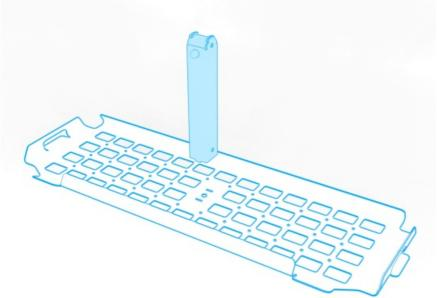
Tighten the thumbscrew from the bottom of shelf.
