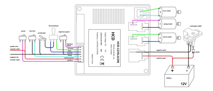
The electronic board is used for kid car, and controls kid car to move forward,move back, swing. Also,can adjust speed accordingly.
