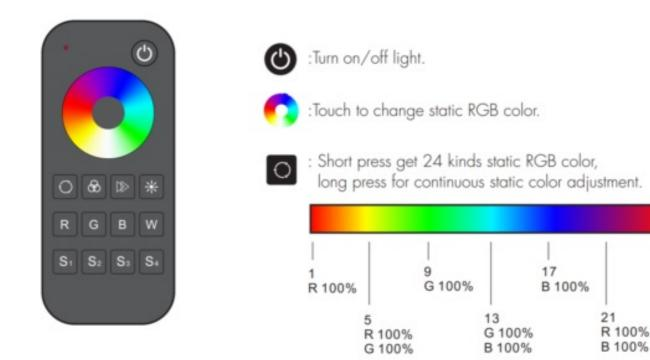
: Short press run next dynamic mode, long press 2s run mode-cycle.
