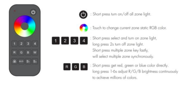
: For RGB light, short press turn on/off white(RGB mix), long press 1-6s adjust saturation continuously, namely change current static RGB color to mixed white slowly. For RGBW light, short press turn on/off W channel, long press 1-6s adjust W brightness continuously, namely change saturation by add white color slowly.
