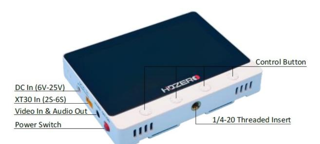
\*When HDZero Monitor is connected to HDZero Programmer APP, Button will be disabled.
