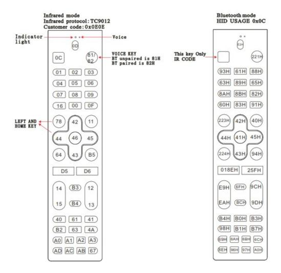
The remote control has two modes: infrared and Bluetooth.
