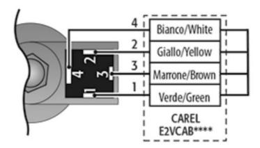
Connection diagram for sensors with control cable for pulse modulating valve — here shown with Danfoss AKV/AKVA
