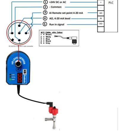
**Note:** The sensor is powered via the M12 plug only. Do not supply the sensor via the cable.
