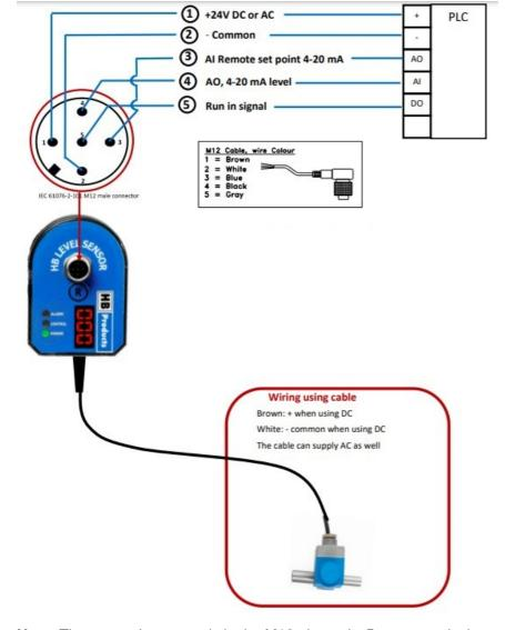
**Note:** The sensor is powered via the M12 plug only. Do not supply the sensor via the cable.
