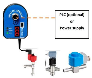
Connection diagram for sensors with control cable for all common stepper motor valves — here shown with Carel E2V
