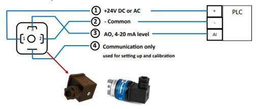
Connection diagram for sensors without control cable.
