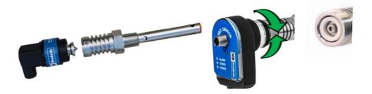
The electronic head is mounted and demounted using either the three pinon screws or a union. The threaded union is mainly used on sensors for low temperature applications. The threaded union should be tightened firmly using a tool to secure good electrical contact and avoid loose connections.
