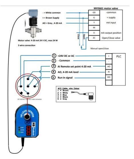
The sensor has a build in controller for a pulse modulating valve. The sensor provides both the analog output via the cable to control the valve. The level measurement signal for the PLC comes via the M12 plug.
