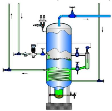
An economiser with an HBSLC connected to the modulating valve, type Siemens MVS661.
