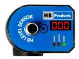
3-digit display: (not available on /S stepper motor control version.) Showing 0...100 % linearly corresponding to 4...20 mA.
