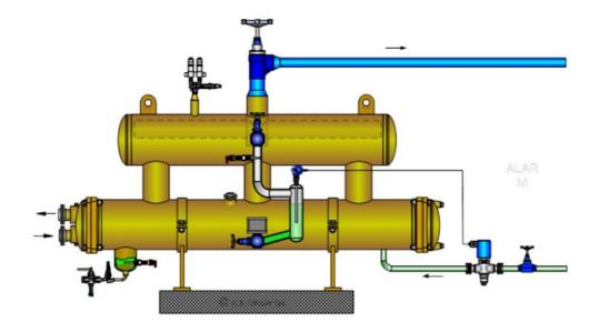
HBSLC connected to a modulating valve – an alternative to low pressure float control.
