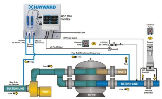
ALL CHEMICALS MUST BE INJECTED DOWN STREAM FROM HEATER & FLOW CELL
