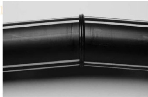
Improper alignment in fusion machine—mitered joint.
