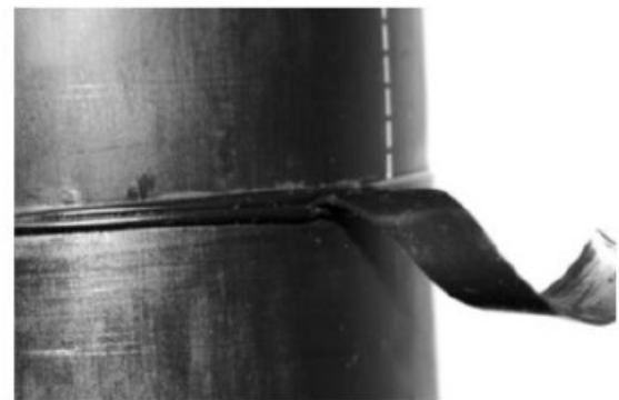
Contamination in joint.
