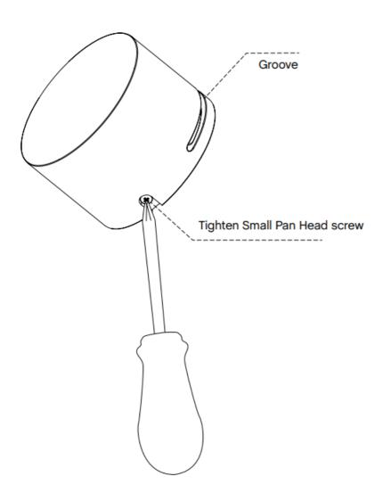
Insert lamp into the wall bracket and push the cable into the groove.
