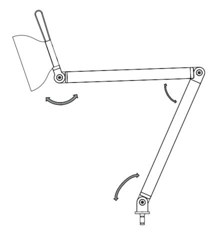
If necessary, the joints can be adjusted using the provided torx tool. Carefully tighten the bolts until the lamp supports itself in any position.
