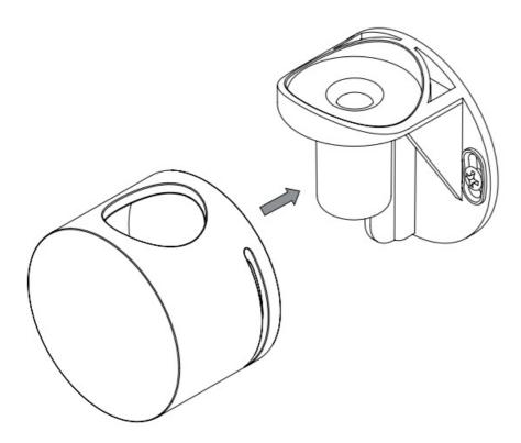
Fix the external plastic cover in place with the provided screw. The groove on the side of the plastic cover provides simple cable management for the wall mounted lamp.
