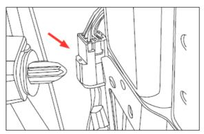
10. Pull the plug toward you. Press down on the plug release and pull to diconnect it from the vehicle.
