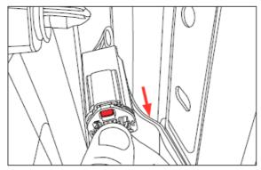
11. Using a grease pencil or painters tape, mark the position on the vehicle where the upper and lower tailgate hinges are mounted.
