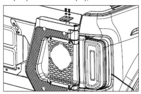
**Note:** The large hole in the bracket is for CB antennas, while the smaller hole can be used to mount a pod light.
