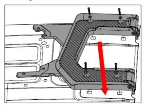
16. While gently holding up the tailgate, slowly close the tailgate. To compensate for added weight of the spare tire, we suggest adjusting the tailgate upward until the latch housing is making contact with the striker. Also, check the gaps between the tailgate and body panels.
