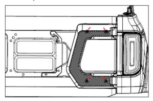
18. Using M6 button head bolt(#8) and washer(#9), attach logo mesh to hinge casting.
