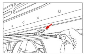
8. Starting near where the wire harness sleeve goes into the side trim panel, lightly pry trim panel open.
