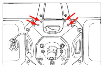
4. Remove the insulation from behind the camera in the tire carrier. Gently, remove the stud plate and camera assembly from the tire carrier. Disconnect the camera from the wire harness. Let 3rd Brake light and wire harness hang below the tailgate. Set OE tire carrier to the side.
