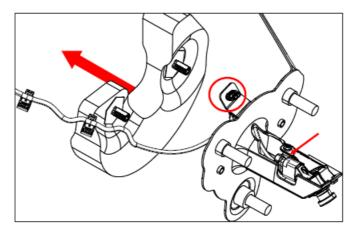
5. Open the tailgate. Using a No. 2 Phillips driver, remove the four plastic rivets next to the tailgate hinge.
