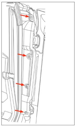
6. Using a 10mm socket, remove the two fasteners near the tailgate hinge. Remove the plastic hinge cover from the vehicle to expose the OE tailgate hinge.
