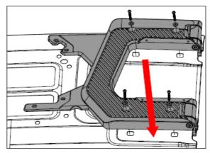
15. Using the marks created in step 11, align tailgate and cast hinge assembly to vehicle. Reusing OE hardware, attach tailgate to vehicle. Ensure the hinge is in the same location as the OE hinge before tightening.
