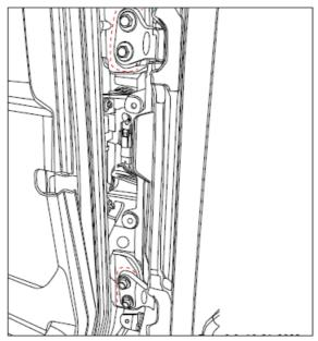
12. Using a 13mm socket, remove the 4 bolts securing the tailgate hinges to the vehicle. Place OE tailgate on table with the outer panel facing up.
