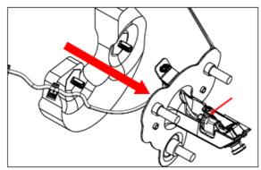
21. Reattach the 3rd brake light to the OE tire carrier. Reconnect plug inside cargo area, tailgate strut, and reattach plastic panels.
