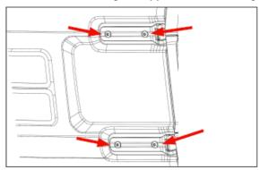
14. Using supplied M8 x 40mm button head(#6) bolt and M8 washer(#7), loosely attach hinge casting to tailgate.
