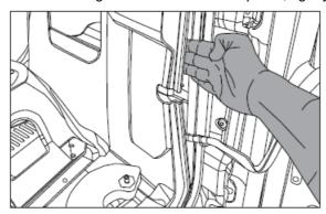
9. With the trim panel lifted, the wire harness plug should be visible. There is a plastic retainer holding the plug to the vehicle. Gently slide a pry tool between the plug and metal body work. Then lift the plug away from the body work.
