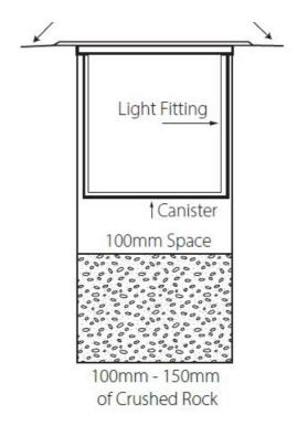
Slight decline on the Ground level to allow for water to run away from fitting
