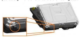
3. Lower back of computer onto Docking Station, ensuring computer properly aligns with the Locator Pin on the Docking Station. With computer seated on Docking Station, **A** apply light downward pressure to the rear of computer and, **B** pull the Front Latching Handle forward until latched.
