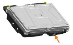
3. Once unlatched grab both sides of computer and carefully lift out of Docking Station, rear end first.
