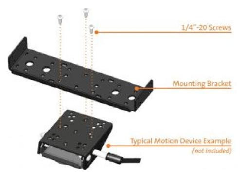
2. Lower the Docking Station to the Mounting Bracket as shown and secure with (4) 1/4"-20 x 5/8" long screws (Hardware Kit Item 3). Torque screws to 80 in-lbs (9.0 Nm)  $\pm$  10%.
