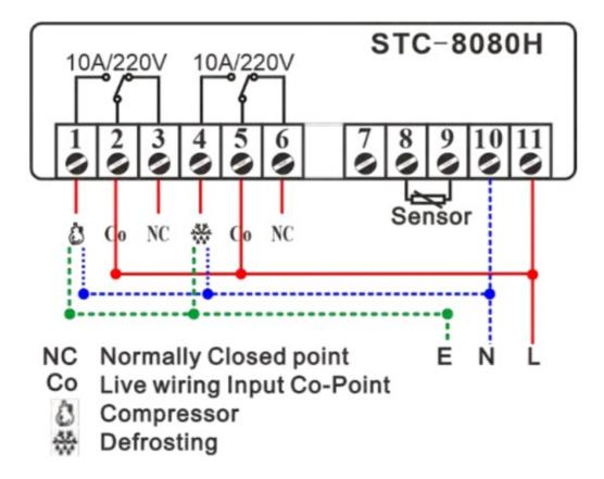
This unit does not output AC electricity; hence you have to wire all live and null wires to each port; you may use the jumper wire conveniently.
