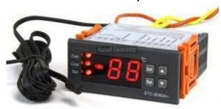
STC-8080H defrosting thermostat with one sensor and two output relays to connect and control the refrigeration and the defrosting unit.
