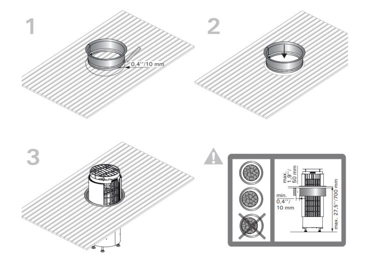
**NOTE!** The benches' distance from the heater can be less than specified in the heater's installation instructions when Harvie HPCU2L/HPCU7L embedding flange is used. See also heater's instructions for installation.
