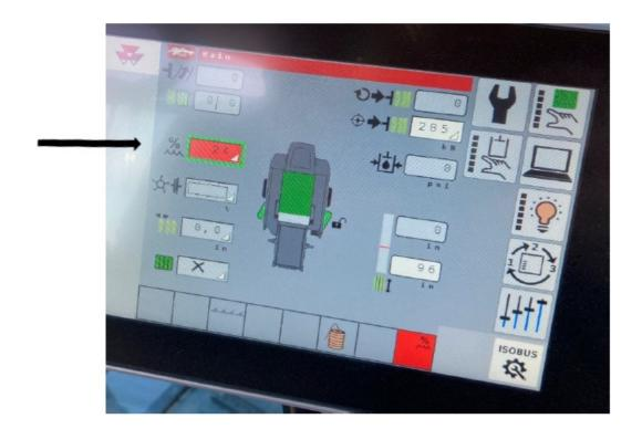
The Error message shown below will come up on the baler run screen when moisture option is turned on but there is no ISO module detected.
