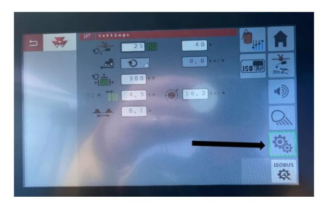
To turn on the moisture system, choose the check mark next to the moisture symbol and select Harvest Tec. Then return to the baler run screen.
