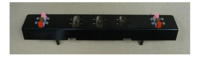
Install the additional manifold block (001-4435NSB) with the six fittings (003-A1414) in place, three on each side,
