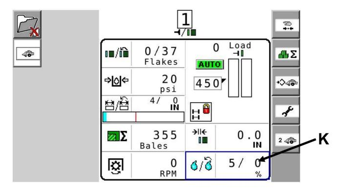
2. To adjust the moisture alarm set point select the box option to the right of the moisture droplets (M) and adjust to the desired moisture limit. To return to the baler work screen, press the baler icon at the top right of the selection menu (N). When the moisture is higher than alarm setting the audible alarm will sound (if turned on) and moisture values on screen will display with red background.
