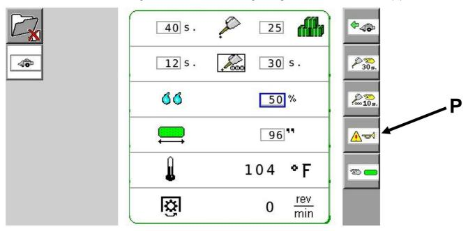
3. The alarm screen should now be displayed. All alarms can be silenced before they are ever heard. This can be done by selecting the **Peak Moisture** icon (Q) and turning the alarm On/Off. To return to the baler work screen, press the baler icon located at the top right of the selection menu. If the moisture is higher than the alarm setting the moisture values will be displayed with a red background but there will be no audible alarm if this is turned off.
