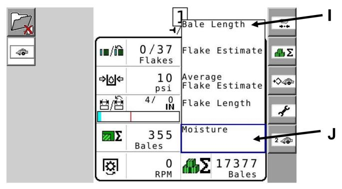
8. The Moisture container will have a red background until HayBoss G2 system is put in Manual Mode or Auto Mode. The two values indicated in the moisture option are as follows: current moisture / last bale average moisture (K).
