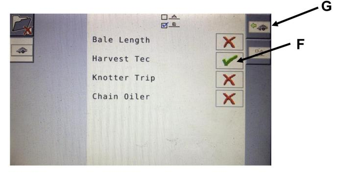
6. The main baler work screen will appear. Select the container (H) where you would like to view the moisture information on the baler run screen. Note: This can be done on the primary or secondary baler work screen. The screen has been or can be customized for viewing containers or options as you would like and as guided in the baler manual.
