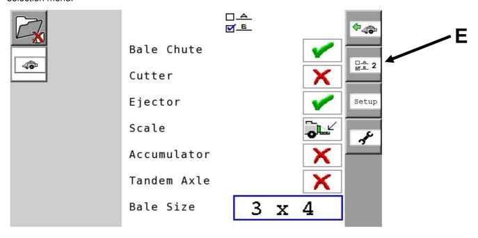
5. The A B 2 screen will appear. The Harvest Tec On/Off selection icon can now be selected. To turn the Harvest Tec Moisture Sensor On (signified by a green check mark) or Off (signified by a red X) navigate to the box and select (F) by pressing the Scroll Wheel. Once the Harvest Tec Moisture Sensor has been turned On/Off you can navigate back to the main baler work screen by pressing the BALER (G) icon on the top right of the selection menu.
