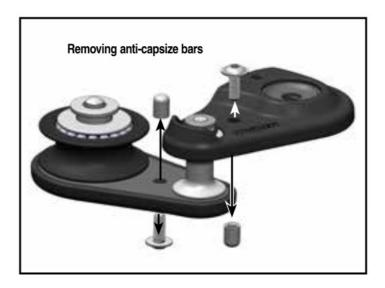
The anti-capsize bar can also be removed if the up-down control is 1:1 and a spliced eye is used, thus avoiding capsizing.
